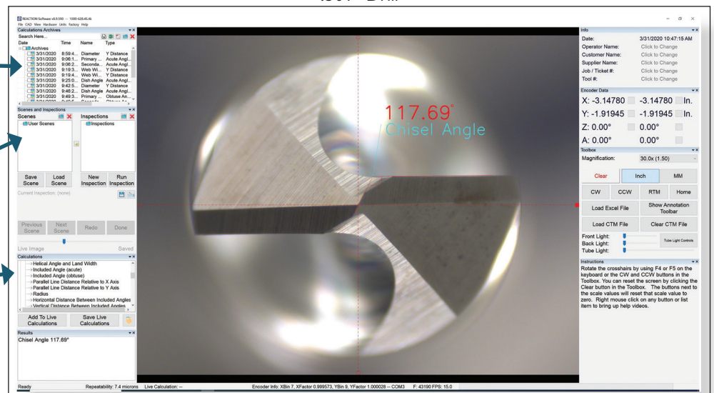
Chisel Angle at 30x zoom
