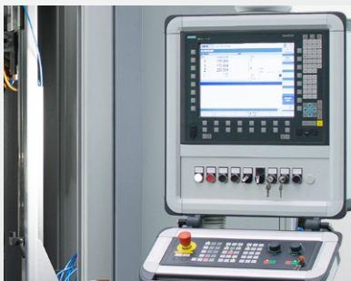
SPE machine with extended swing type operator panel, 15" screen.
