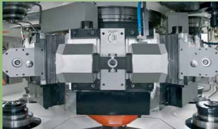
Self-centring chuck with CNC automatic jaws rotation for 4-side machining
