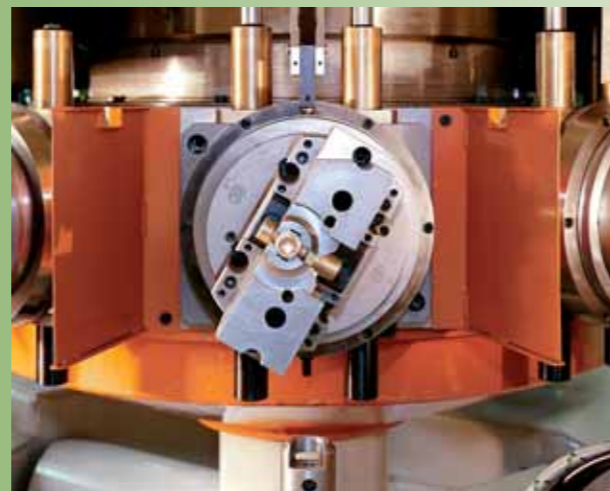
CNC rotating clamping fixture with rotation of 360° for 5 or more side machining
