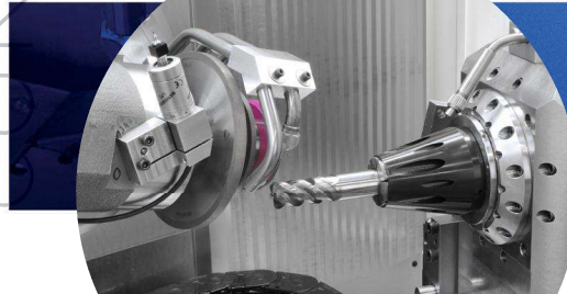
6-axis kinematic - constant grinding point for relief operations on ballnose, radii and form tools - Maximum freedom in axis movements due to the 6-axis design and the total symmetry of the spindle axis (A)
