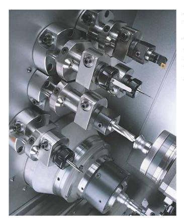
An additional 5 back-boring stations, 2 of which are live, further enhance the machine's flexibility.
