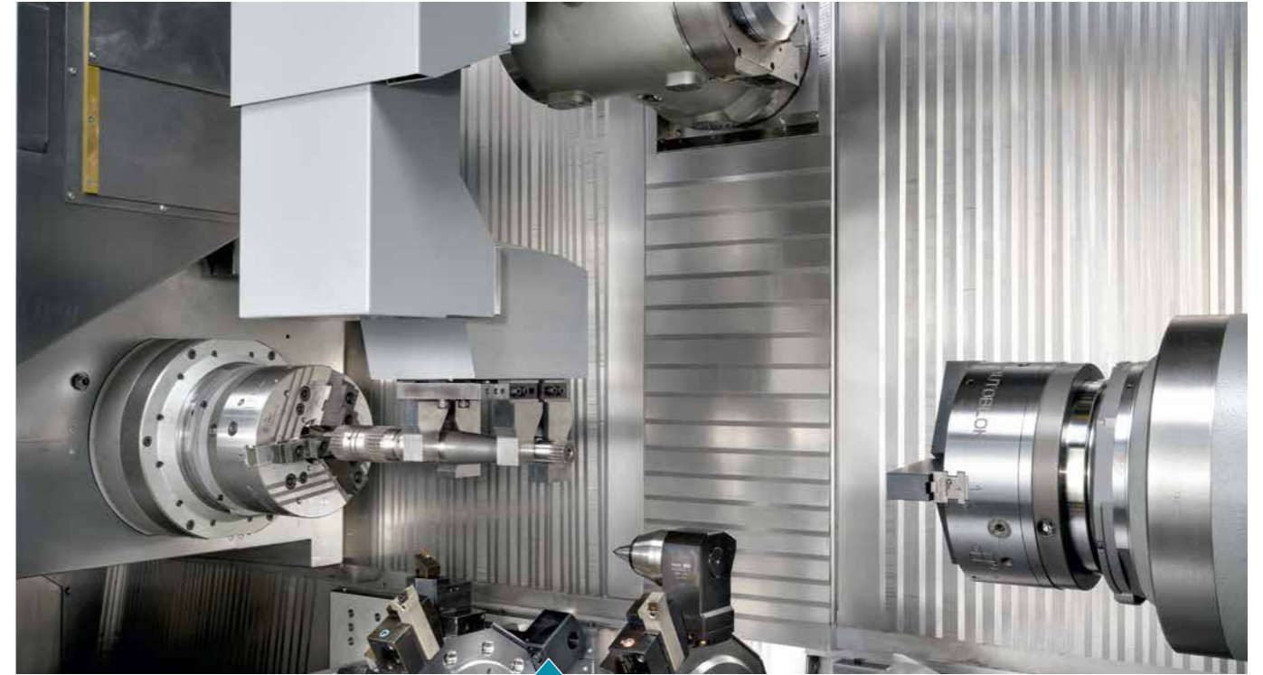
Removal of finished parts (or feeding) using a workpiece-specific gripper for shaft parts or flange parts
