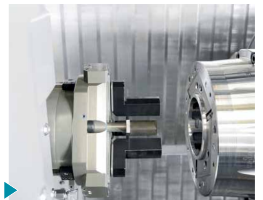
3-axis workpiece handling for flange parts
