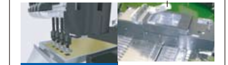
Placement speed 0.65s/chip 4 components x two-time batch transfer by high-flexibility heads (LS8 nozzle)
