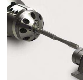
Square clamping with tailstock for taps & reamers
