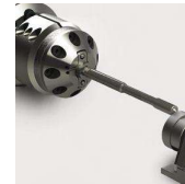
Square clamping with tailstock for taps & reamers
