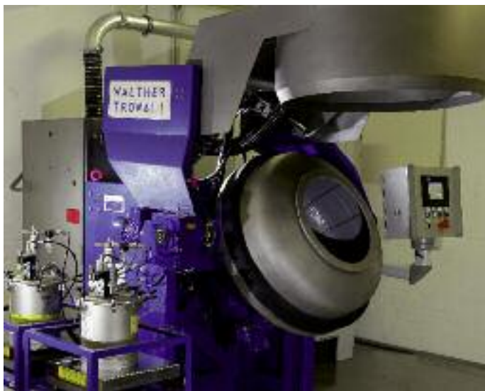
Rotamat R 90 C with opened cover
