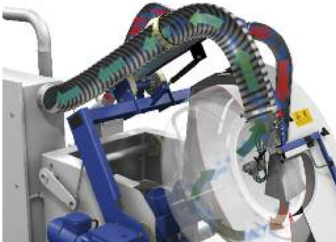
Inlet and exhaust air system; red arrow: heated inlet air, green arrow: exhaust air
