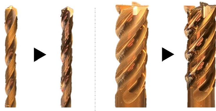
Left : Before removing droplets, Right : After polishing
